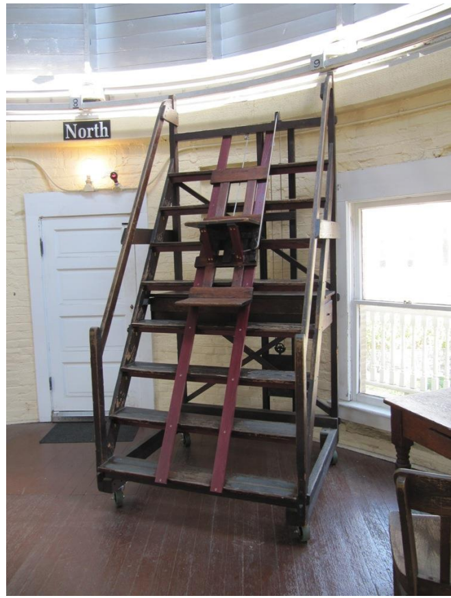
The observer's "chair." To raise the chair, push the chair up. To lower the chair, while sitting on the chair pull DOWN on the rope at your LEFT side.
