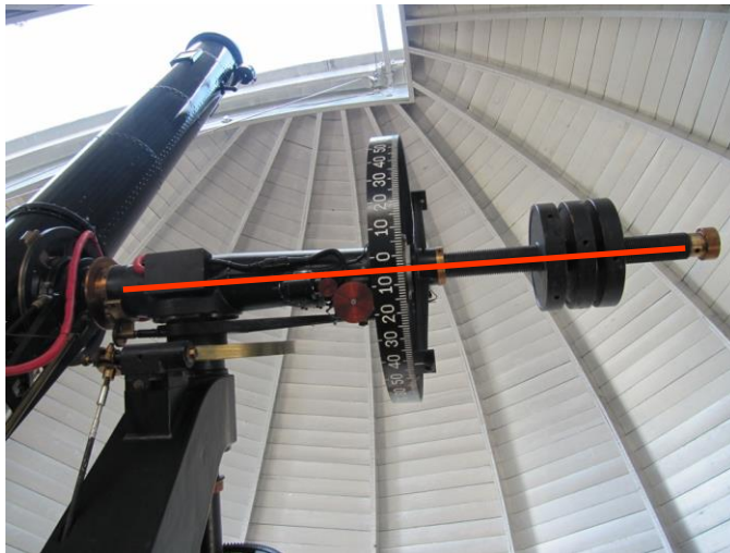
The Declination Axis (red line) and Setting Circle
